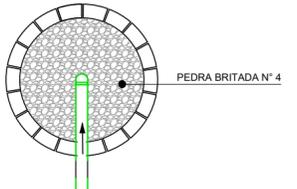
**PLANTA BAIXA - SUMIDOURO SEM ESCALA**
