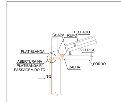
DETALHE-PASSAGEM DO TQ PELA PLATIBANDA SEM ESCALA
