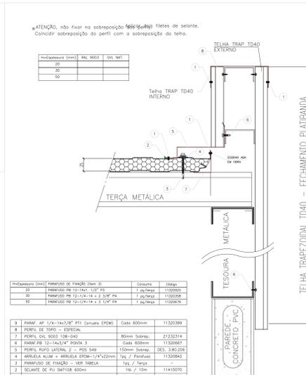
6 DETALHE FECHAMENTO PLATIBANDA SEM ESCALA
